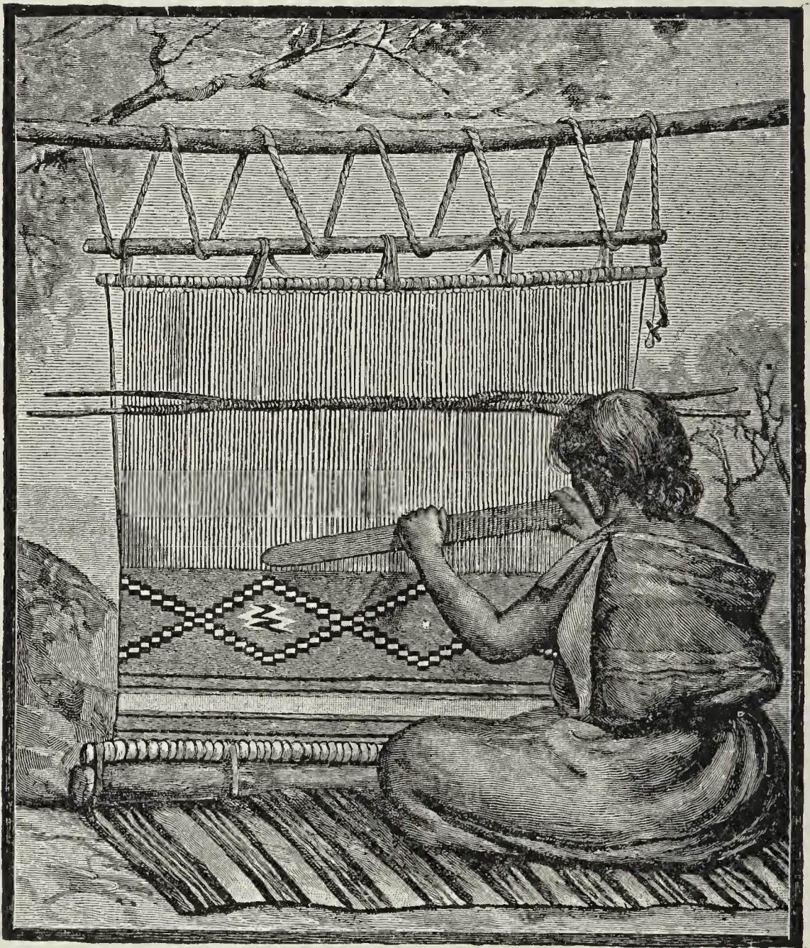
Fig. 77.—Ordinary Navajo blanket loom. The heald, to which the warp threads of the lower shed are attached, and the batten or sword-shaped stick for pushing down the weft, are well seen. (After Matthews.)
